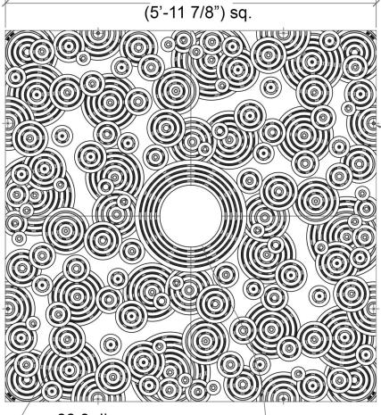
attatches to frame (x8) w/ 0.25 - 20 UNC button - head tamper - resistant s.s screws
